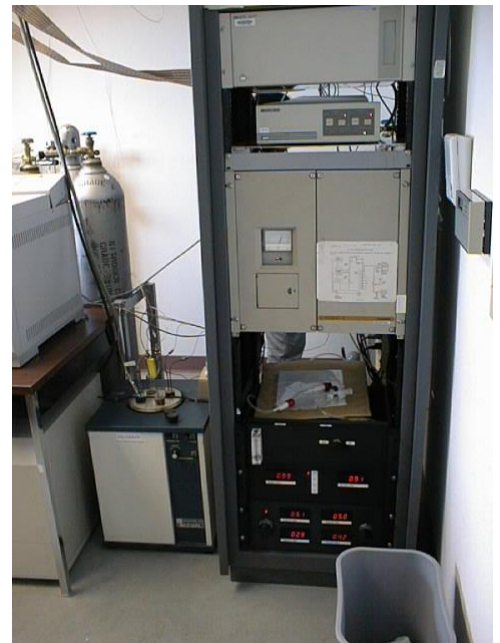
Figure 4. non-dispersive infrared (NDIR) analyzer
